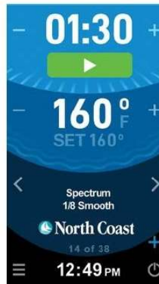
Home screen with factory presets of thermoplastic sheet recommendations.
